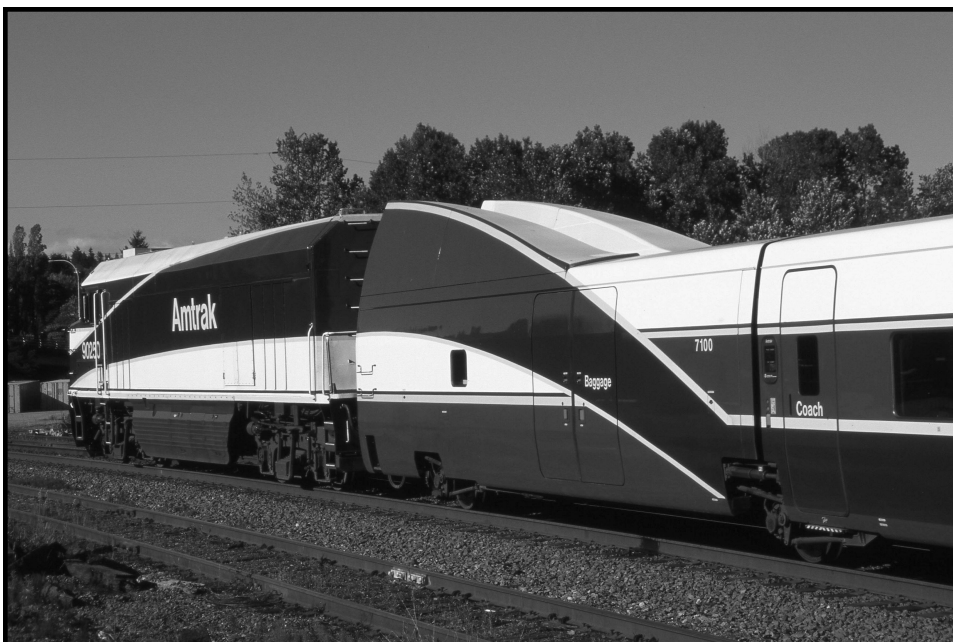
The “batwings” of Series 6 baggage car 7100 swoop up to the roofline of Non-Powered Control Unit 90250, which trails the southbound train in New Westminster on June 24, 2000. Note the single wheels on each articulated car. (Photo by Ian Smith)
