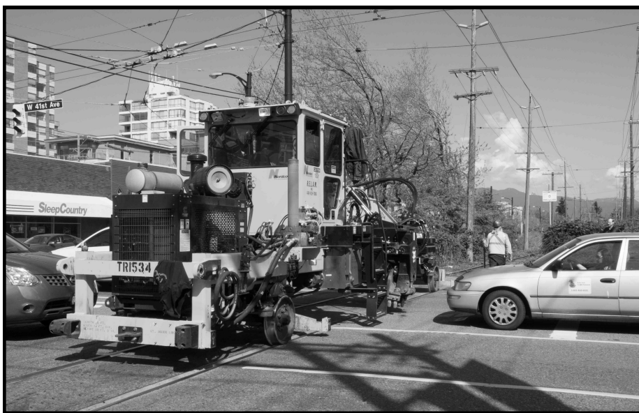
A Nordco tie exchanger ties up traffic on busy West 41st Avenue on April 8. Work will include upgrading the crossing control gear here. (Photo by Ian Smith)
