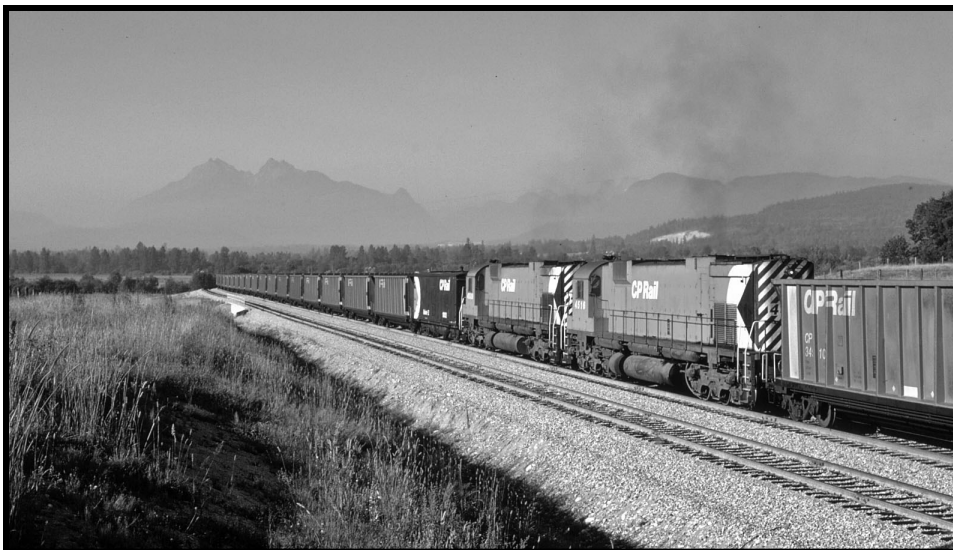
Operating as mid-train remote slaves, MLW M-630 units CP 4516 and 4509 are positioned ahead of the robot car in this westbound CP coal train on the CN Rowlison Subdivision in Langley, B.C., on August 22, 1970. (Photo by Dave Wilkie, WCRA Archives)
