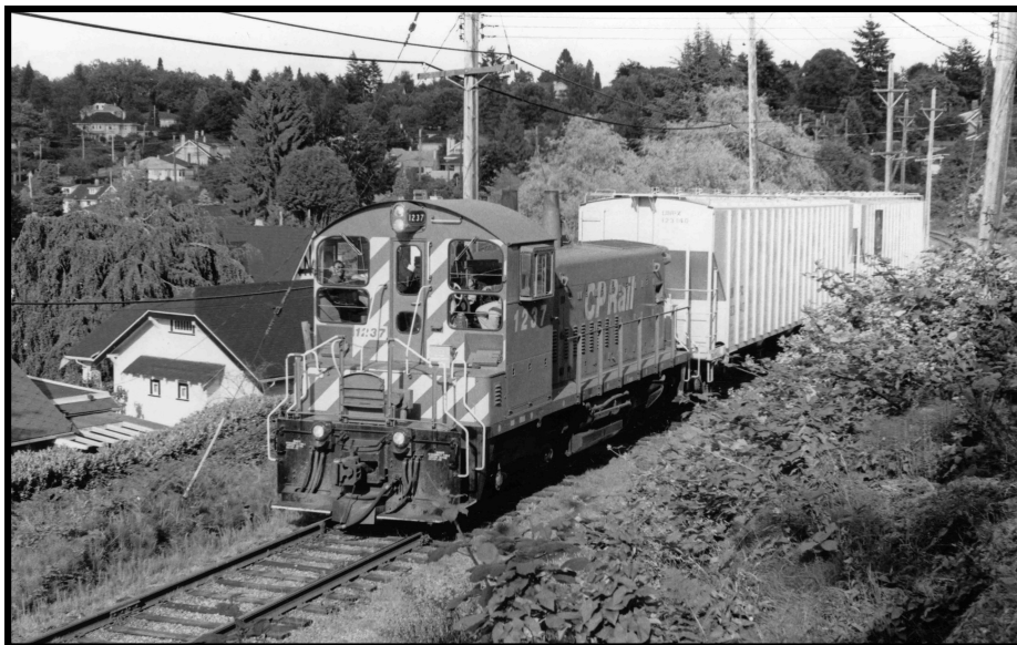
About to cross West 25th Avenue, running southbound, CP 1237 has just charged up a 2.5% grade after descending a 2% slope from West 16th Avenue, on July 27, 1992, with parallel Arbutus Street to the left. Below, 1237 climbs a 1.5% grade, after crossing West 33rd Avenue on June 1, 1992 on its way south, as it wends its way past houses on the city's affluent west side. No "wrong side of the tracks" here!
