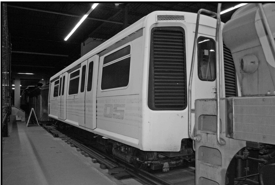
Innovia ART 100 car 2135 is seen in the warehouse of the Canada Science & Technology Museum, Ottawa, in 2012. It was one of two cars, numbered BC-1 and BC-2, used for the SkyTrain demonstration service in Vancouver in 1983. (Photo by Paul Bown)
