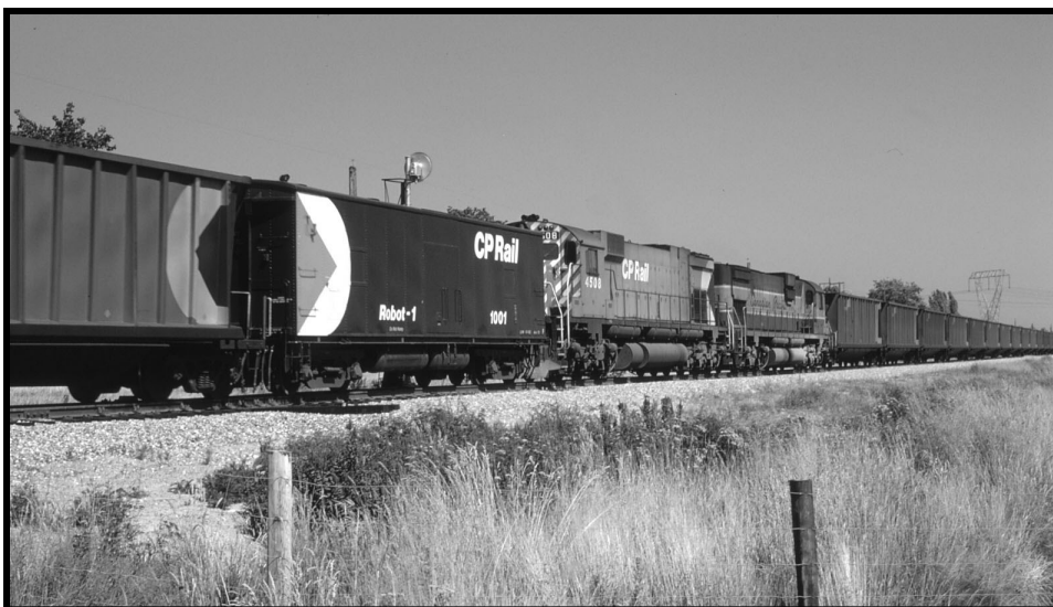
Robot car 1001 trails remote locomotives 4501 and 4508 in an eastbound empty coal train at Mile 6.4 of the BC Harbours Board Railway (now the BCR Port Subdivision) on August 22, 1970.
