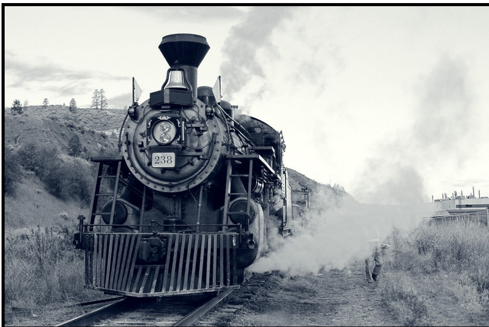
The most prominent features of 2141's disguise as 238 were a diamond smokestack and a pilot of vertical bars added in front of its solid pilot. (All photos by David J. Meridew)
