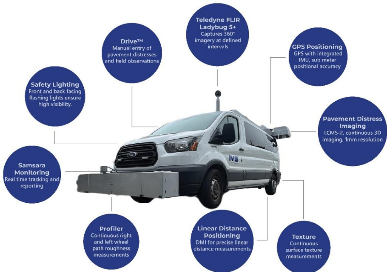
Figure 4 LCMS-2 RST data collection vehicle (IMS, 2023).
