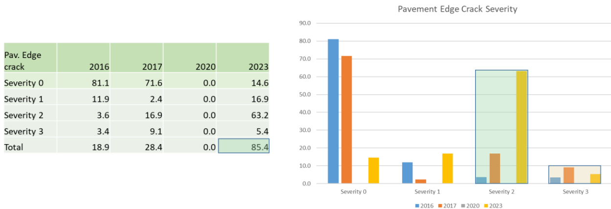
Figure 28 Pavement Edge Cracking Severity in percentages All years - Comprehensive table and bar chart showing Severity distribution across all years
