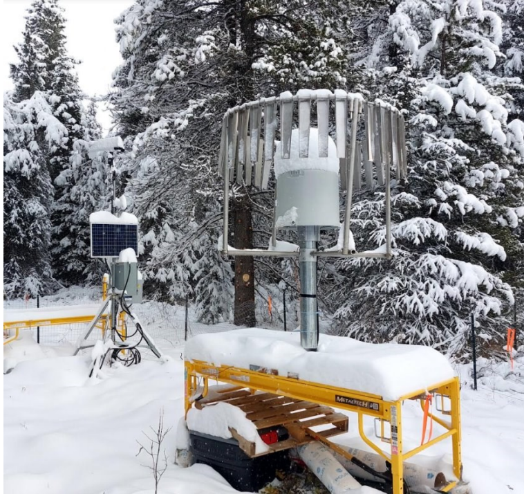
Figure 4.1: This year-round meteorological station, photographed on 9 October 2024, monitors meteorological and hydrological conditions in the G aat Héeni Watershed. It records total precipitation (mm), wind speed ( \text{m s}^{-1} ), air temperature ( ^{\circ}\text{C} ), relative humidity (%), and atmospheric pressure (hPa), with data collected by an OTT Pluvio 2 , RM Young wind monitor, and ATMOS-14 sensor. A 50-watt solar panel supplies power, and an XLINK500 datalogger with Iridium telemetry transmits data remotely. A nearby OTT RQ-30a radar sensor provides measurements of river discharge ( \text{m}^3 \text{s}^{-1} ), level (m), and velocity ( \text{m s}^{-1} ).
