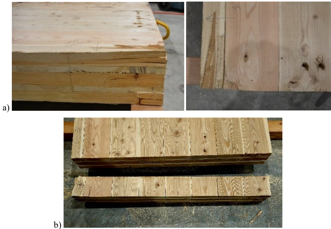
Figure 29 a) Damaged panels, b) trimmed CLT panel
