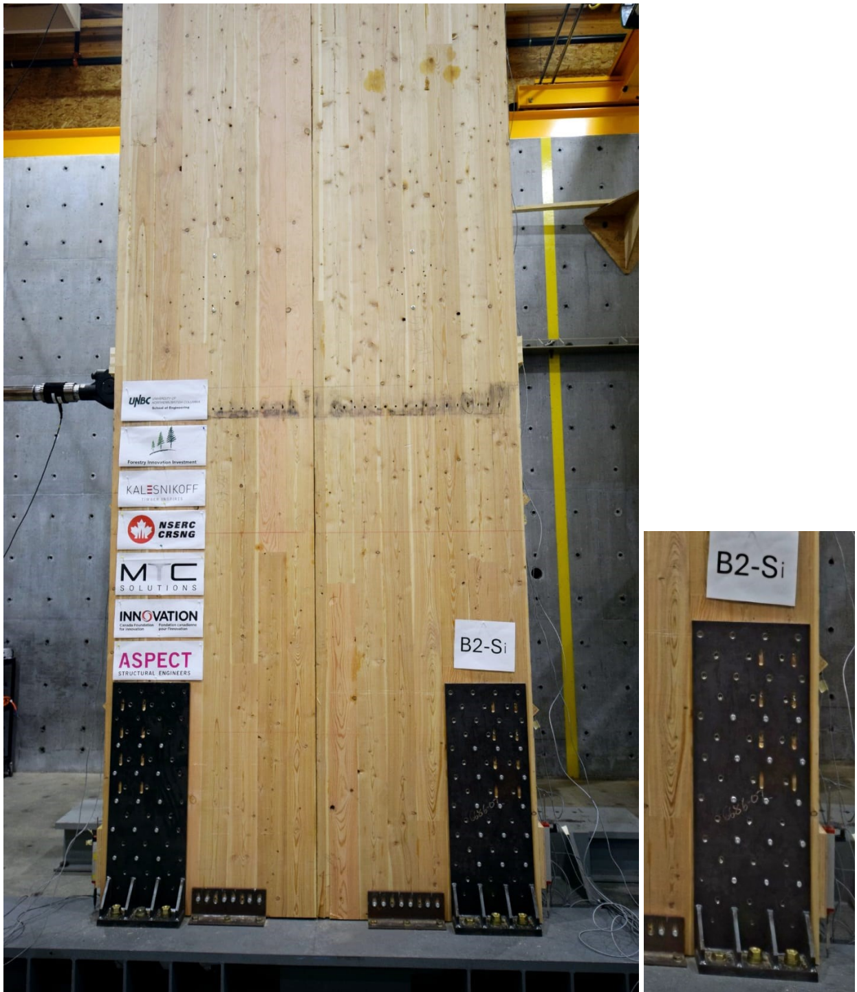
Figure 47 B2-Si with lower number perp. screws HD
