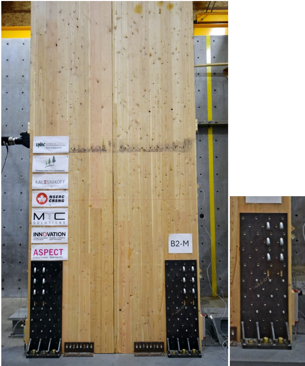
Figure 46 B2-M with mixed screws HD
