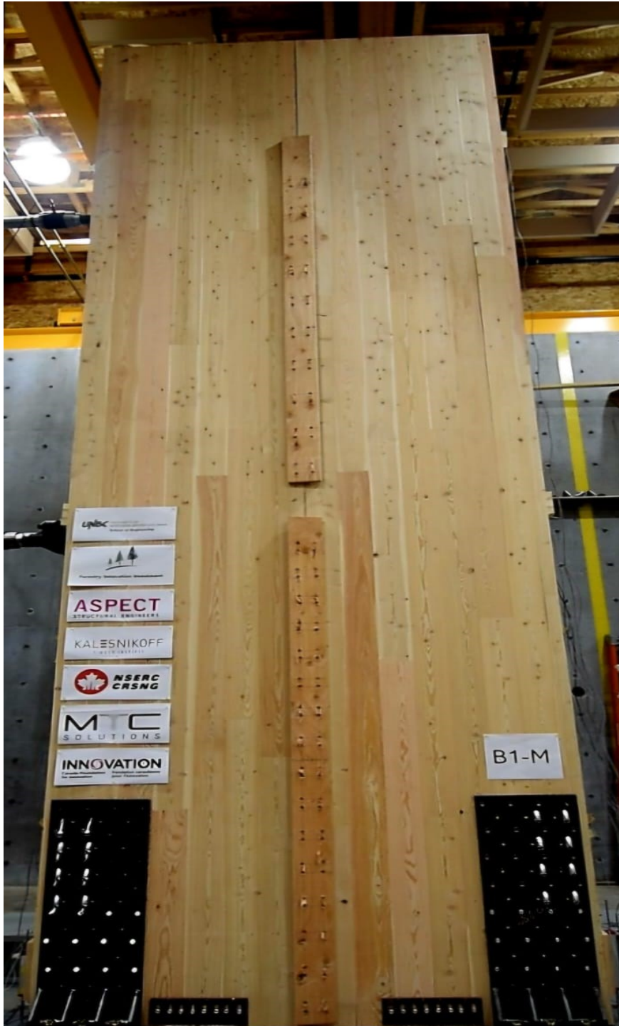
Figure 44 B1-M with mixed screws HD
