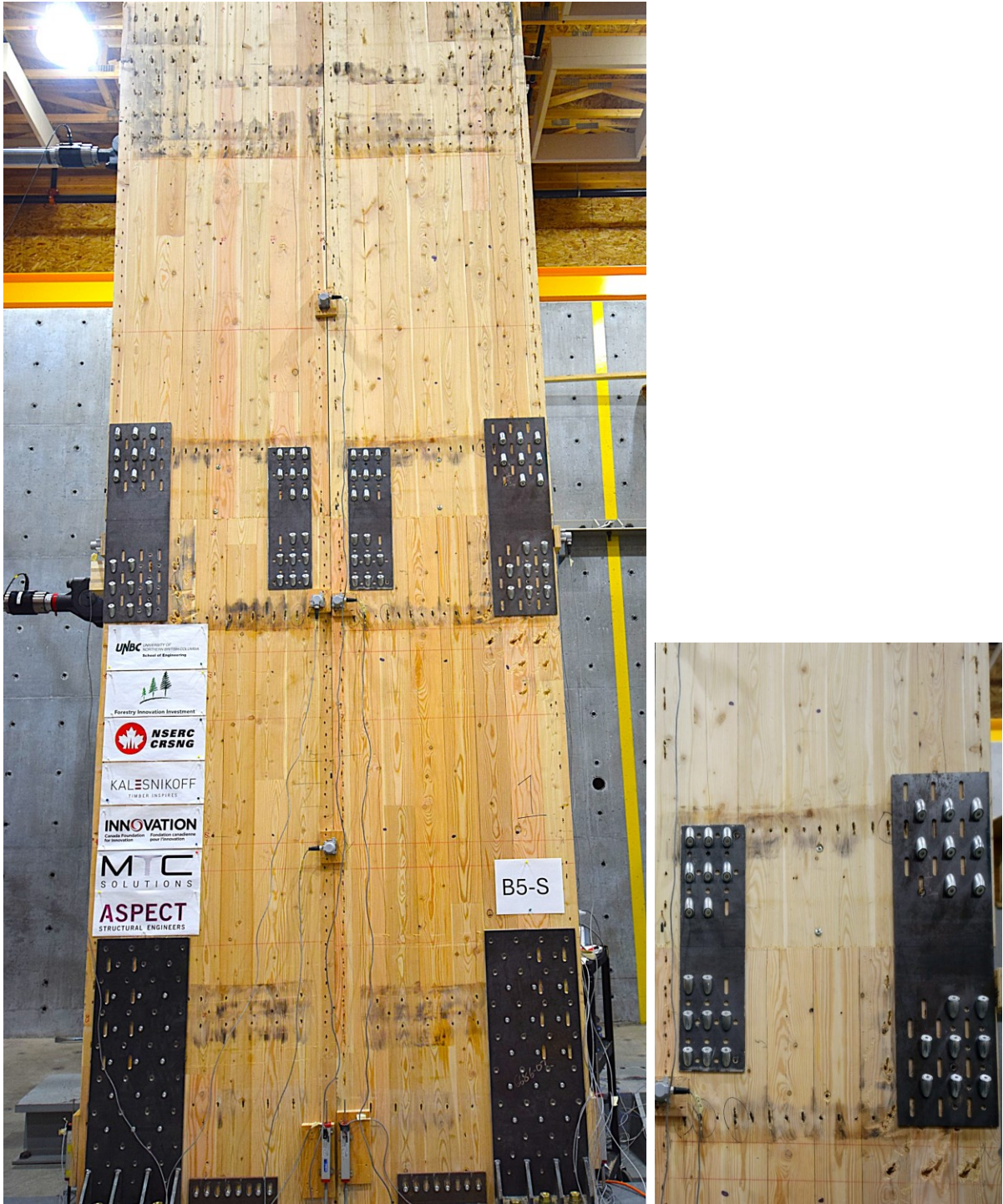
Figure 51 B5-S with tension straps
