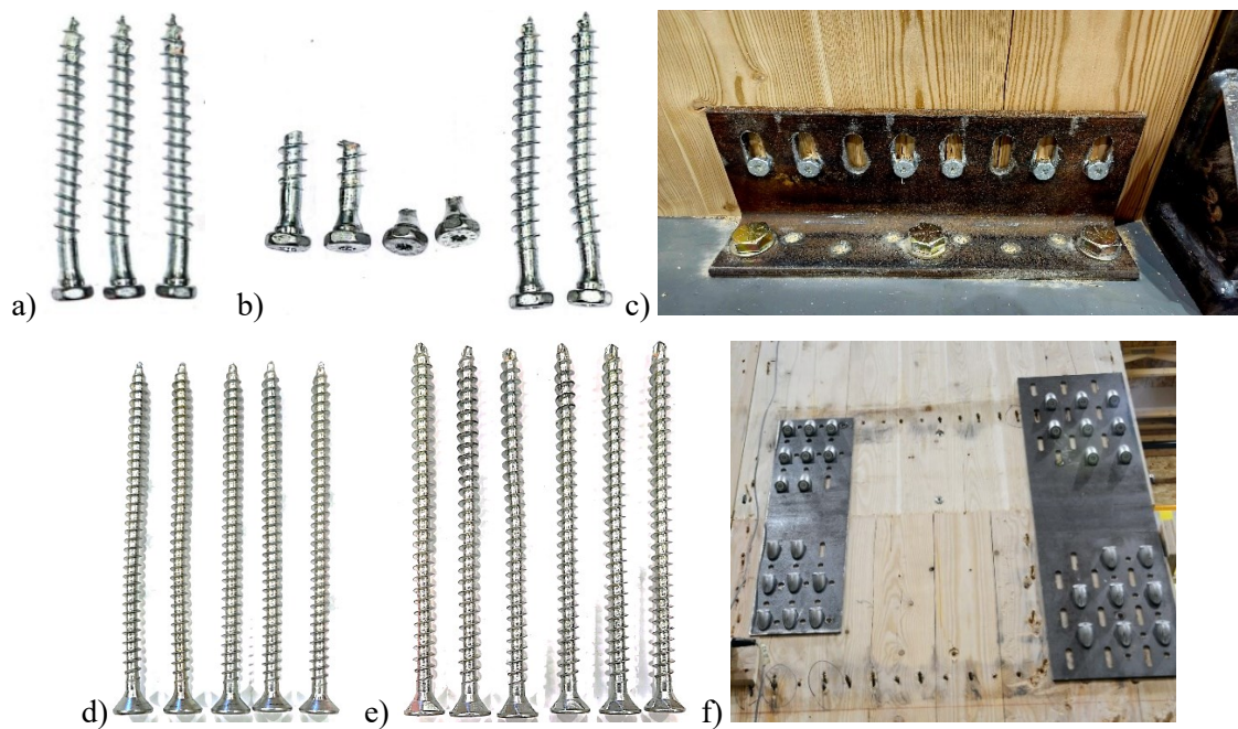
Figure 28 a) SB screws, b) ledger screws, c) SB, d) inner TS screws, e) outer TS screws, f) inner and outer TS after test
