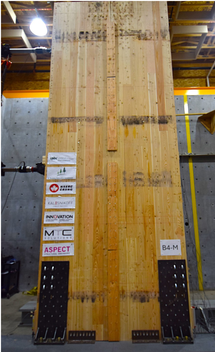
Figure 50 B4-M with mixed screws HD
