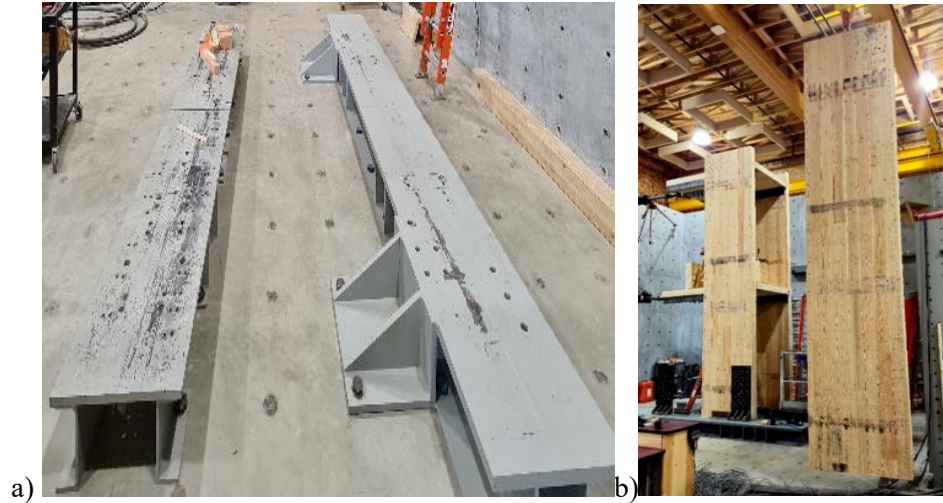
Figure 12 Assembly of house: a) steel base fixture; b) installation of panels on base fixture
