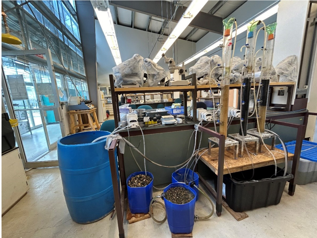
Figure 3.2: Full biofiltration-based water treatment setup
