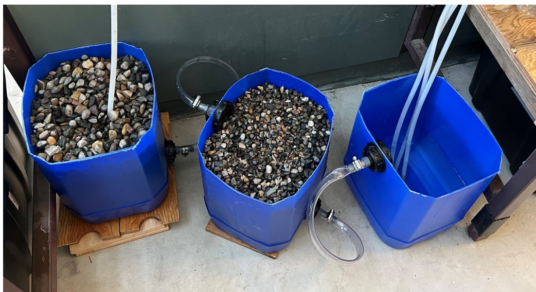
Figure 3.1: Roughing filter set-up
