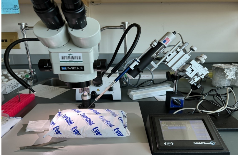
Figure 2.2 Microinjection set up using UltraMicroPump3 with MICRO2T and Microliter syringes (Hamilton; World Precision Instruments). Emerged adult mountain pine beetles ( Dendroctonus ponderosae , MPB) are placed on an ice block, immobilized with entomology forceps, and injected between the second and third abdomen compartments.
