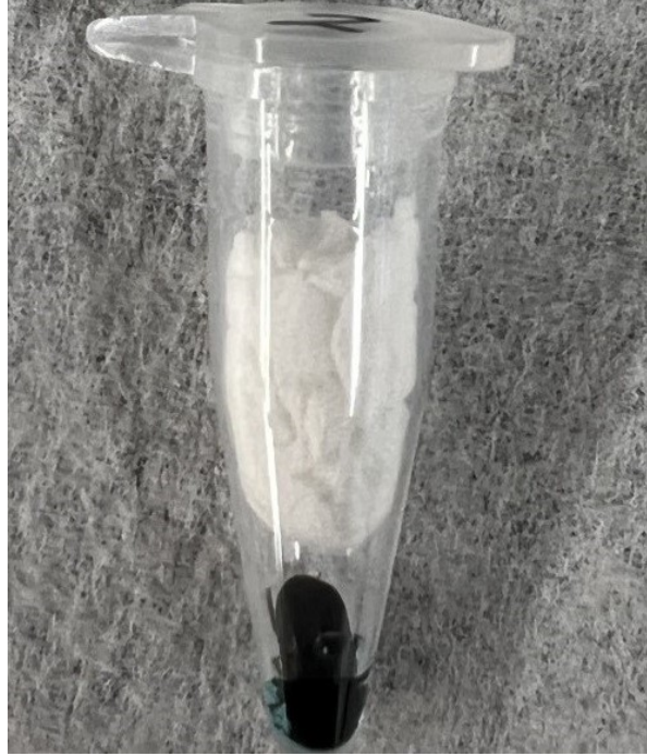
Figure 3.1 A submerged adult mountain pine beetle ( Dendroctonus ponderosae , MPB) in blue-dyed 1% sucrose solution. Beetles were submerged in liquid to the posterior end of the pronotum for 12h.
