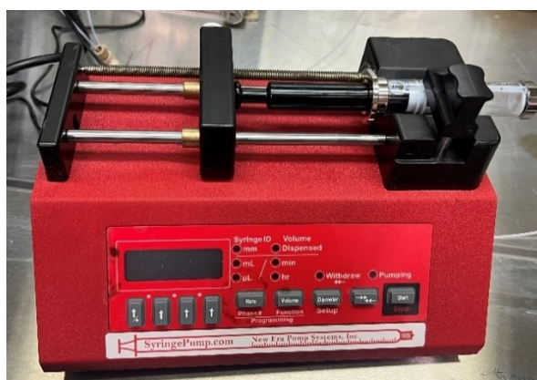
Figure 4: The syringe pump used in the laboratory (New Era Pump Systems Inc.).
