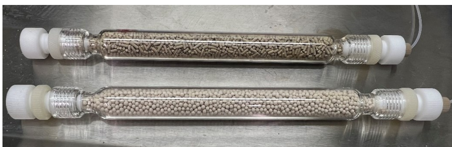
Figure 7: Molecular sieve columns (4A and 3A - top to bottom) used in the laboratory setup.
