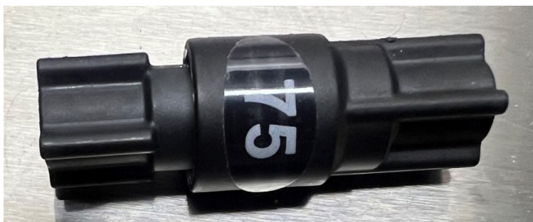
Figure 6: Back Pressure Regulator (IDEX Health and Science) Used in the Laboratory Setup (75 psi).
