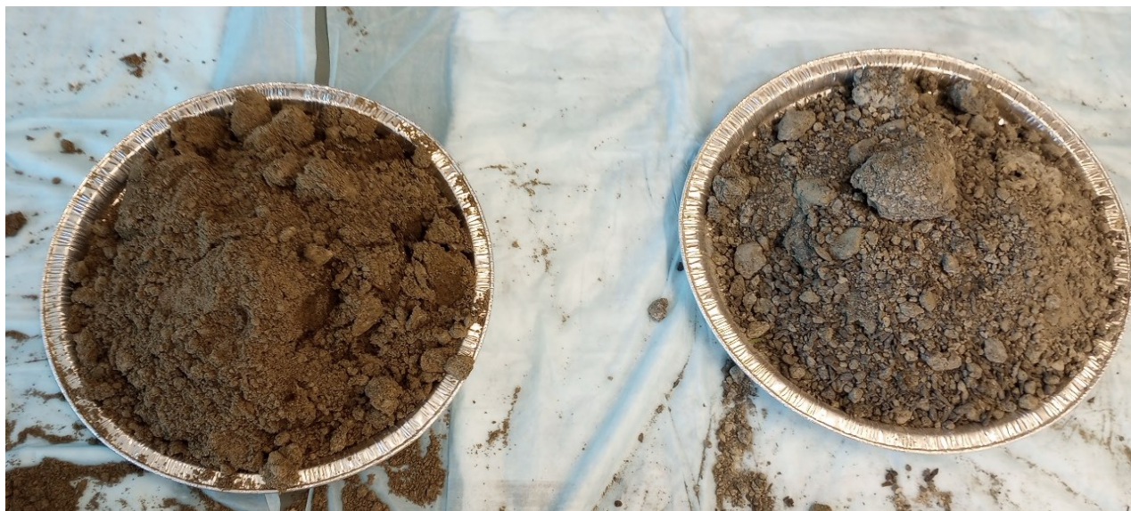
Figure 33. Examples of the aggregates observed within the compost technosols. The pan on the left contains aggregates from the 12.5% compost treatment and the pan on the right shows a sample from the negative controls.
