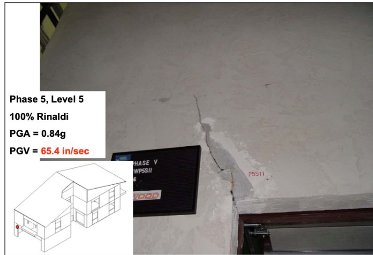
Figure 9 Cracking and Spalling of Stucco at the Corner of Garage Wall Opening (Christovasilis et al., n.d., 2009)
