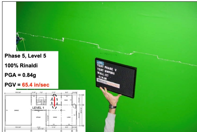
Figure 13 Horizontal Cracking of Gypsum Wallboard (Christovasilis et al., n.d., 2009)
