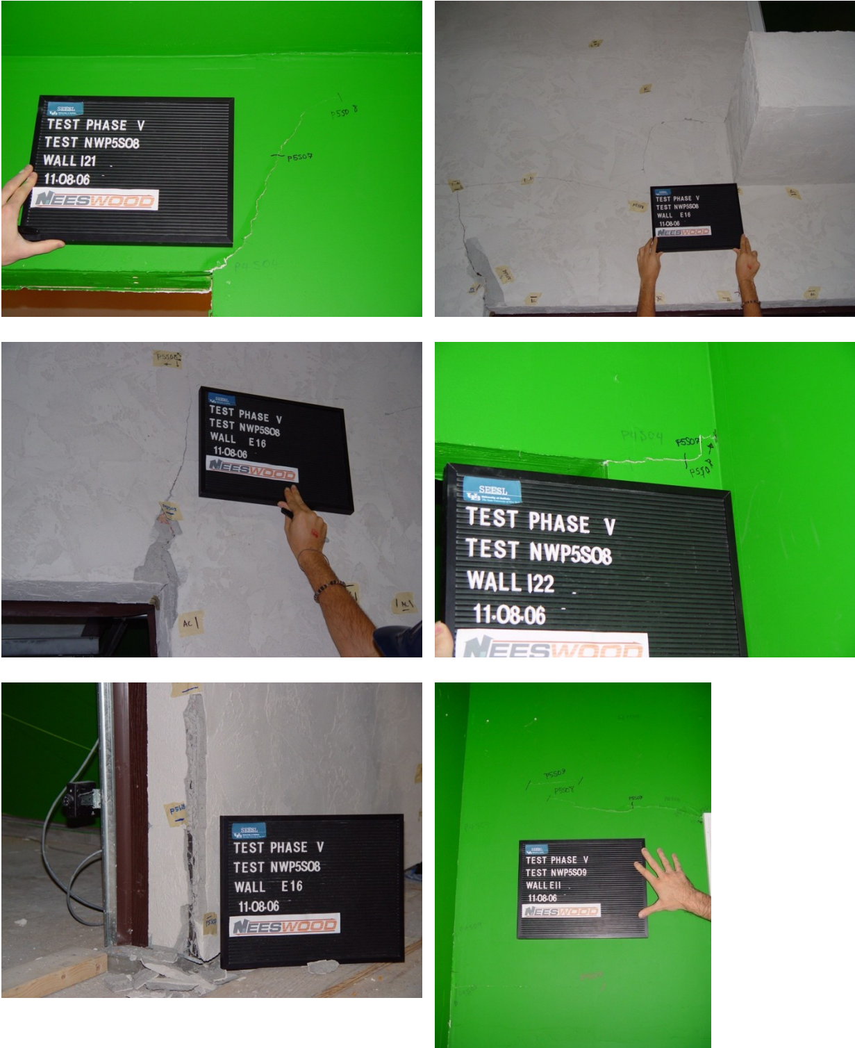
Figure 43. Observed damages for the NEESWood benchmark test after Phase 05 Test 08
