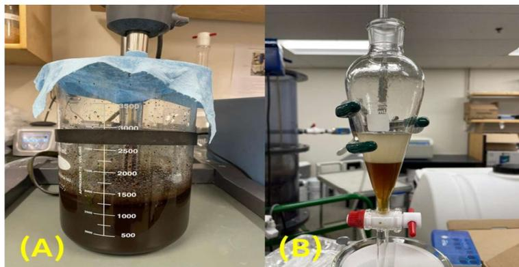
Figure 3.2: Images of (A) prepared oil-water emulsion and (B) oil extraction step
