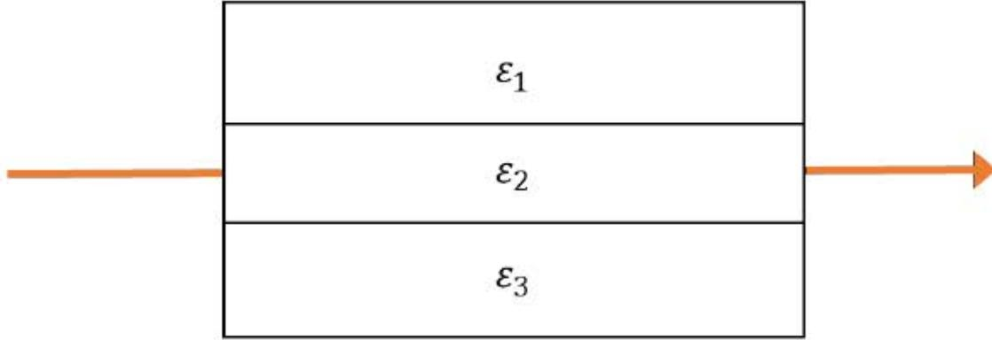
Figure 4.1: Pictorial representation of a three-phase striped composite medium, where red arrow indicates the direction of the electric field.
