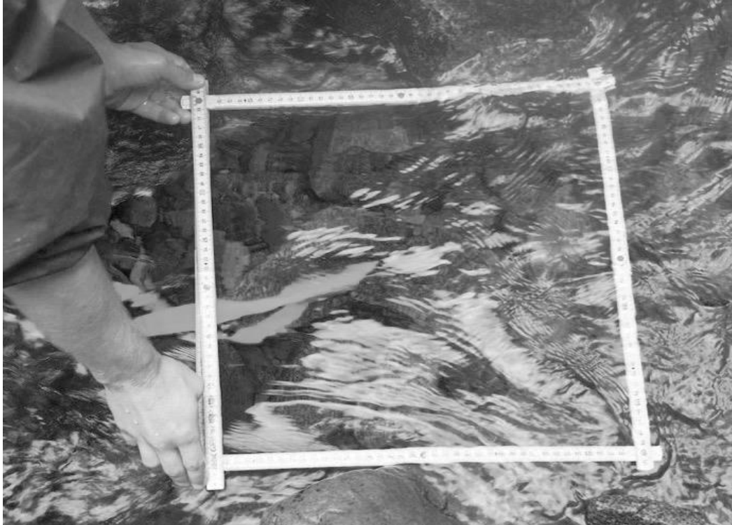
A3.2. Fine-scale habitat assessment array used to measure percent cover of substrate sizes over the point of capture for A. truei larvae in northwestern British Columbia, Canada.
