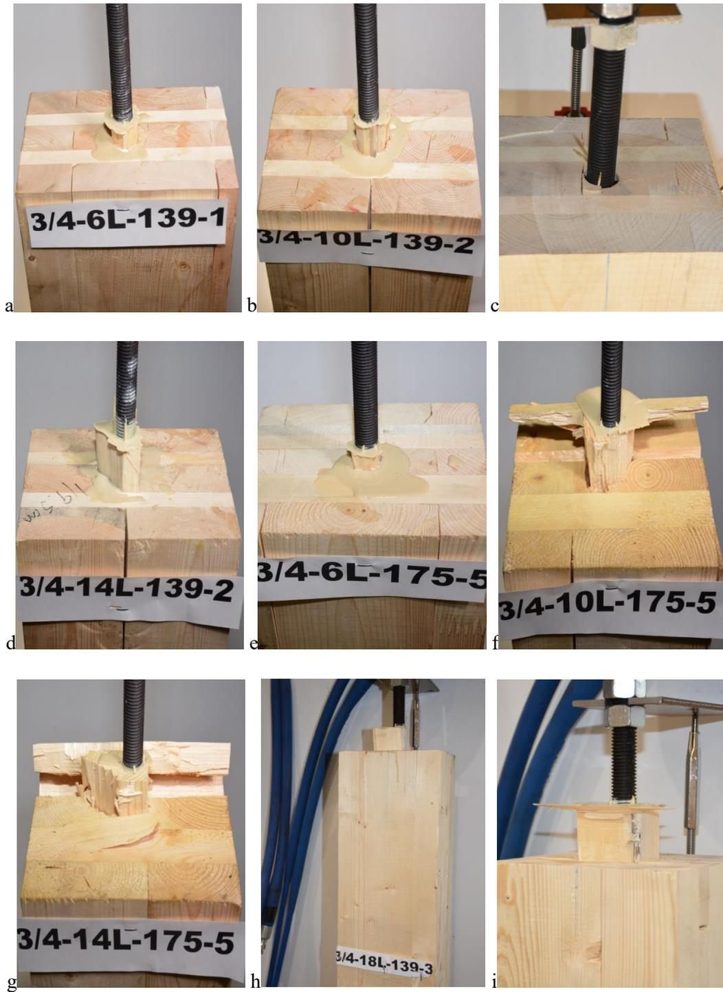
Figure 4.3: Typical failure modes for 19.1 mm GiR par. to the major strength axis
