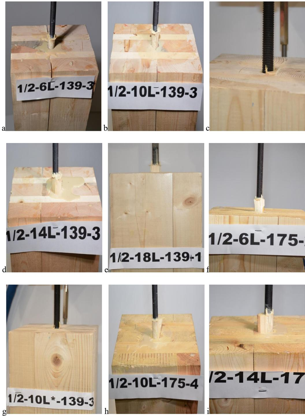
Figure 4.2: Typical failure modes for 12.7 mm GiR par. to the major strength axis
