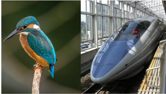
*Figure 3 kingfisher in the left and fast train on the right which inspired the shape from the bird<sup>3</sup>*
