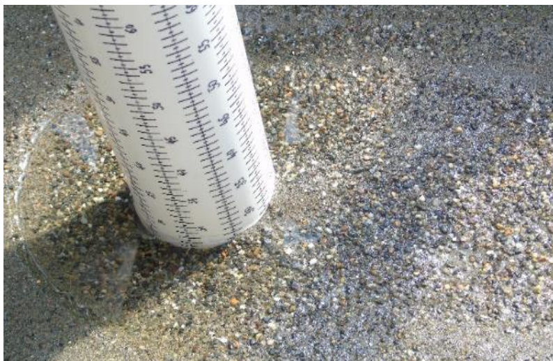
Figure 3-16: Armour layer developed around the 17-cm-pier
