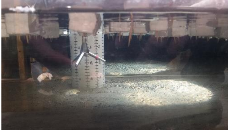
Figure 3-30b: The ADV measurement around the bridge piers under rough ice-covered condition
