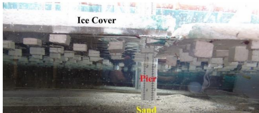
Figure AI-3a: Side view of scour hole around the 11-cm-bridge pier under rough ice-covered condition
