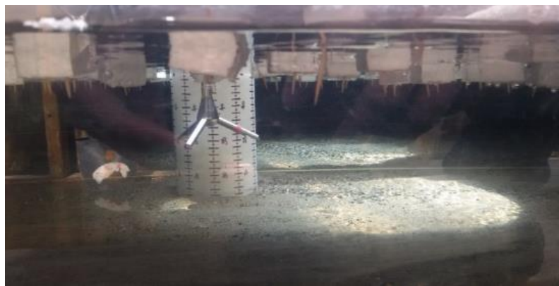
Figure AI-10: 10-Mhz Acoustic Doppler Velocimeter in use to measure the velocity field around bridge piers under rough ice-covered flow conditions
