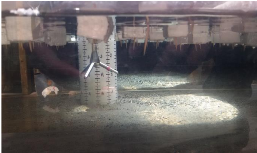
Figure 2-6: 10-Mhz Acoustic Doppler Velocimeter (ADV) in practice used to measure velocity field around bridge piers
