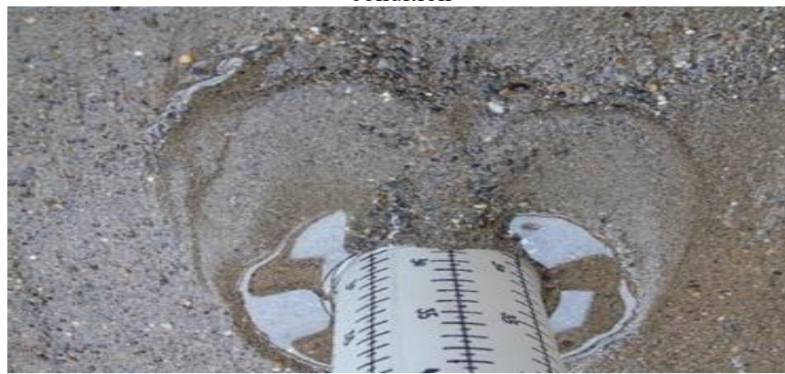
Figure AI-3a: Side view of scour hole around the 11-cm-bridge pier under rough ice-covered condition
