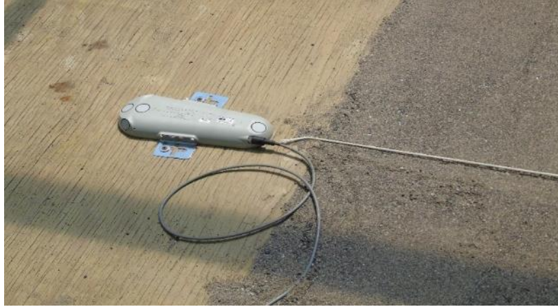
Figure 2-5: The SonTek-IQ used to collect flow (area-velocity) and volume data
