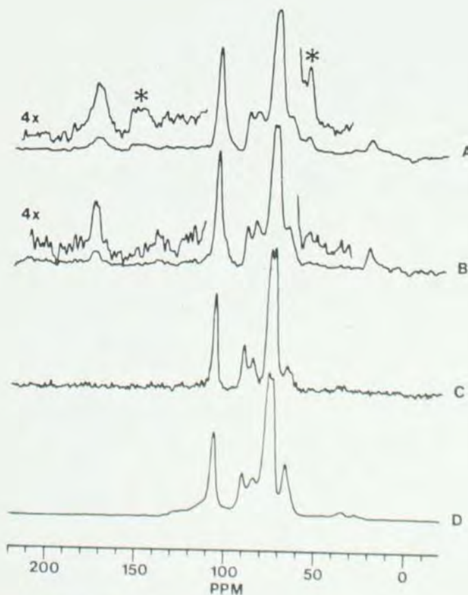
Figure 3. 13 C CP/MAS NMR spectra of Esparto grass derived samples. Spectrum A corresponds to the native material after ethanol/benzene washing. Spectrum B is chlorite holocellulose. Spectrum C is holocellulose extracted with 1% NaOH. Spectrum D is a commercial Esparto grass pulp.
