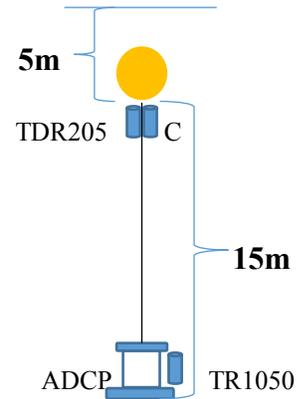
**Figure 3.2:** Diagram of DFO mooring setup.
