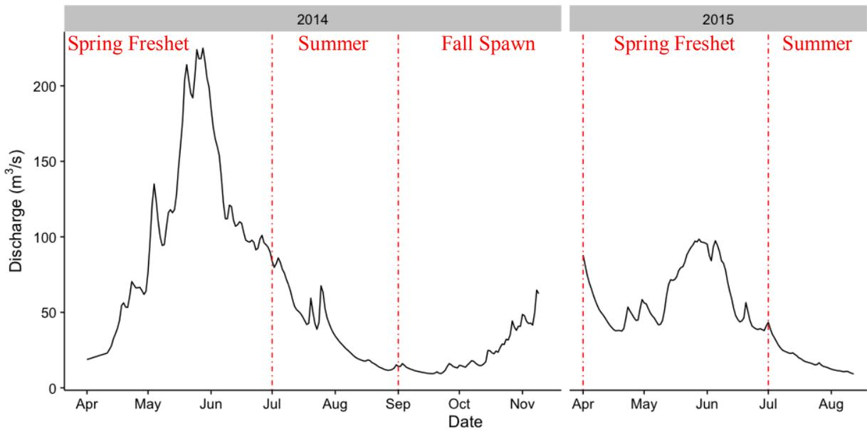
**Figure 2.2:** HFR hydrograph, data taken at the river delta every five minutes. Red lines designate sampling periods in 2014 and 2015 (Environment Canada).
