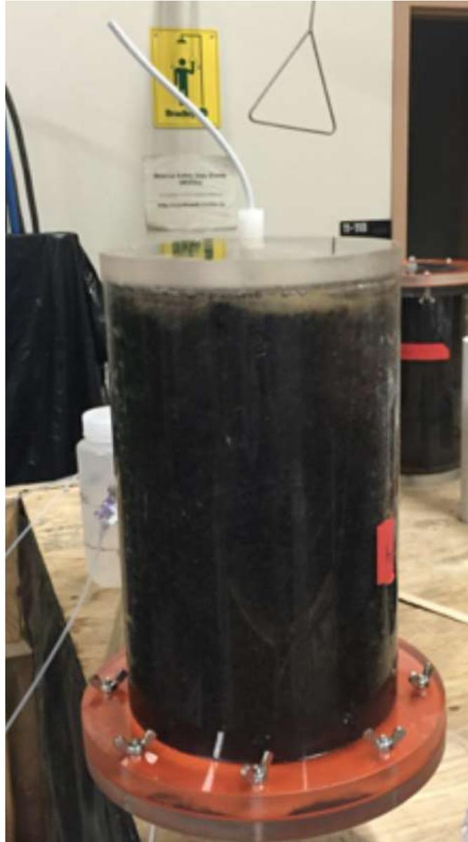
**Figure 2.4:** An inverted column during maintenance - changing a leaking influent hose (on the bottom). Note the 3.18 mm x 3.18 mm (1/8" x 1/8") compression fitting on the column bottom. This allowed tubing to be firmly sealed to the column bottom. A similar fitting was attach attached to the effluent (top) side.
