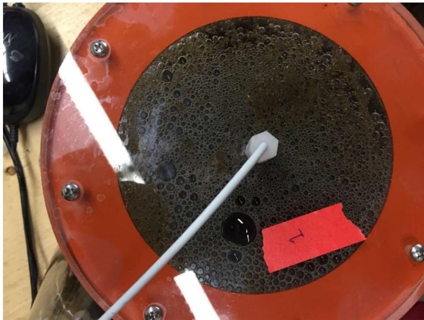
**Figure 3.1:** Gas bubbles building up at the top of column 1. Rapid discharge of gas at specific periods during the column operation (at higher than average liquid flow velocities) may have contributed to organics plugging the column discharge port.
