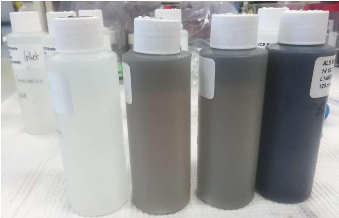
**Figure 3.5:** Week 4 water quality samples (filtered through 0.45  $\mu\text{m}$  filter). Front four samples were collected, from left to right, from column 2 (CMWR only), 5 (hay, sawdust, and CMWR), 3 (hay and CMWR – results not included in thesis), and from 1 (hay and CMWR).
