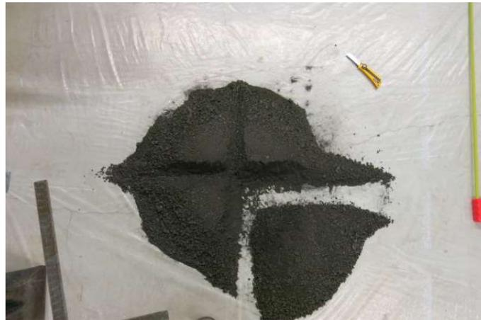
**Figure 2.7:** Cone and quarter method in progress.
