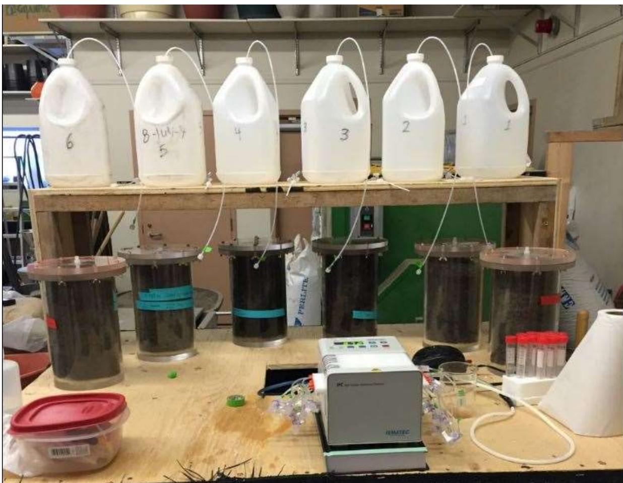
**Figure 2.6:** Experimental setup – configured for normal flow through operations (columns were not yet connected to overflow collection jugs)
