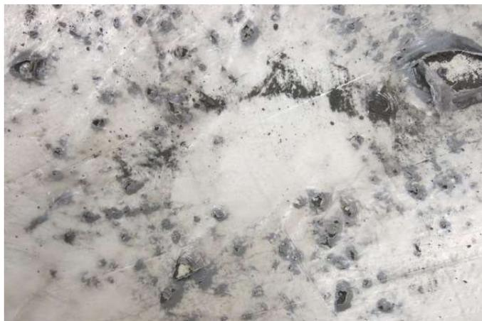
**Figure 2.8:** Residual fines left on the plastic sheeting after a cone and quartering event.
