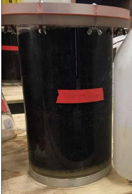
**Figure 2.1:** Column with 1 cm layer of Ottawa Sand overlain by organic amendment mixed with CMWR.
