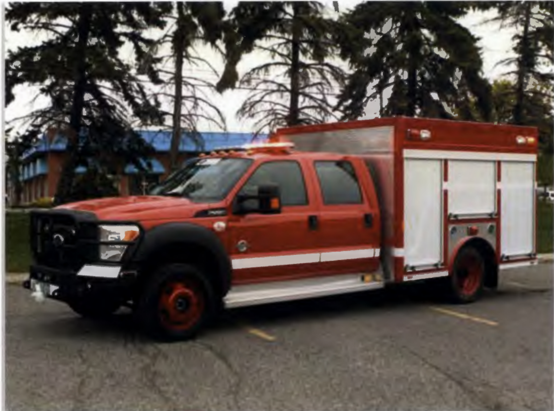
Figure 3: Example of a fire truck body on 2012 Ford F-550 diesel chassis
