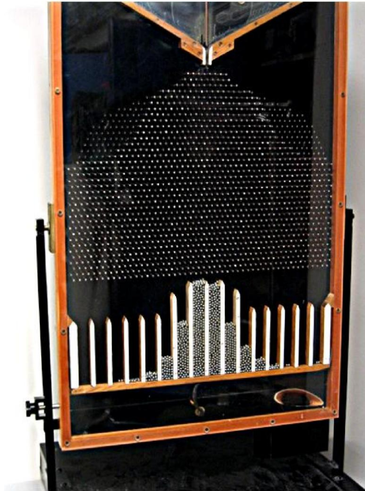
Figure 7: Device for demonstrating the binomial or normal distribution. Individual-level predictions are virtually impossible, but some statistical summaries can be predicted.
